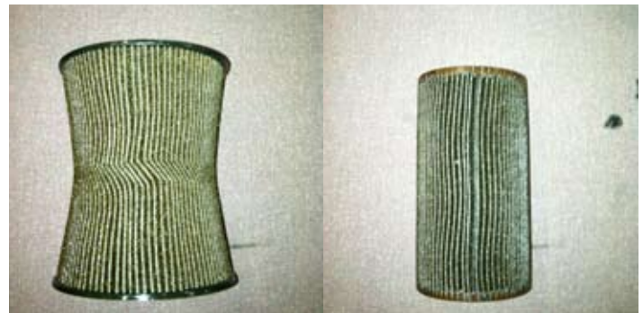
Collapsed oil filter
