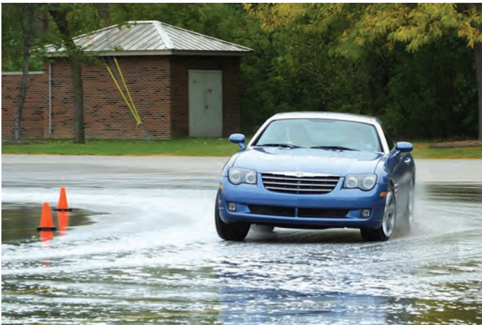
Slippery when wet. Skid pad practice with soap and water from a fire truck.
