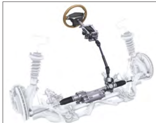
Electric Rack and Pinion Steering. Note motor is mounted parallel to the Pinion for “Bottom Up” control of motor.
