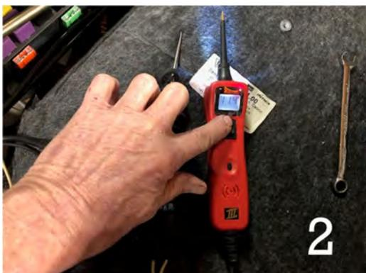
3. You can induce power or ground into a circuit with the push of a button. Here again if the circuit is shorted to ground, the breaker will "Pop" saving your circuit. Most will show a red power or green ground when you activate it.
