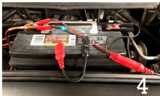
5. When hooking up, use the ground lead by the Power Probe unit. This is necessary!
