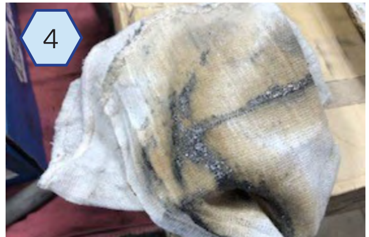
Here's some of the bearing material that was left in the IMS Bearing (shaft) Tube that we were able to recover.
