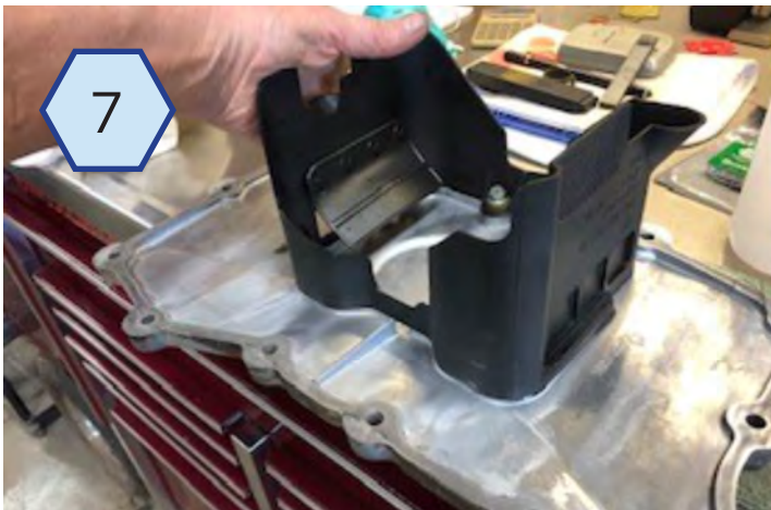
Note the side baffles in the oil pan. They prevent the engine from being starved of oil during hard turns and cornering.
