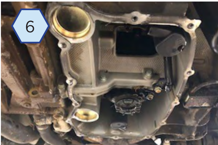
With the oil pan off, the inside of the engine looks pretty clean, almost no sign of debris.
