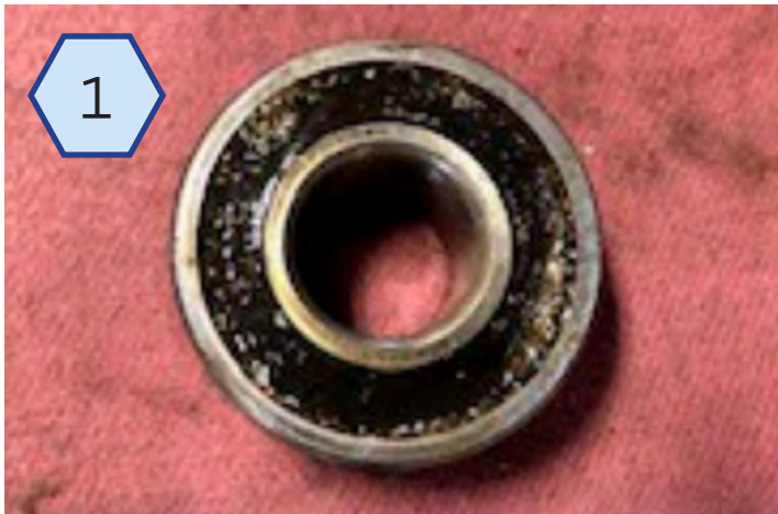
This is why we recommend replacing the IMF bearing if it has never been done. We caught this bearing just in time.
