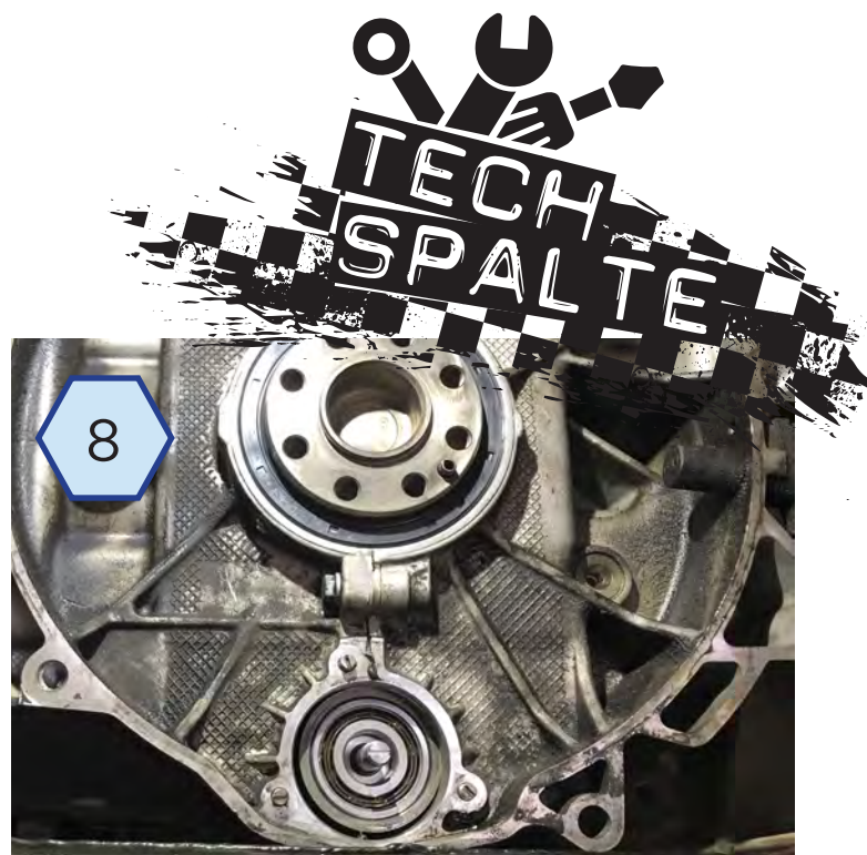
Note the new bearing installed into the IMF shaft tube.
