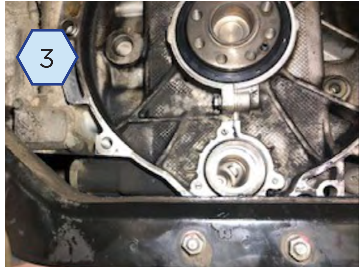
Note the IMS tube which runs from the front of the engine to the back. Oil only seeps into this tube, so fortunately almost all of the debris is still trapped inside.
