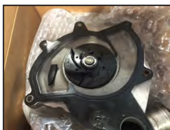
Catastrophic Water pump failure. Not only are the impellers broken, the impeller wheel was spinning freely on the shaft. This new pump had just been installed.
