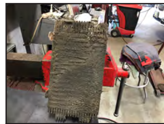
This is the front oil cooler from a 1970 S 911. It was completely packed with what appears to be body undercoating from years earlier.
