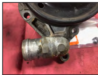
Note the stain on the hose neck caused by coolant leaking under the pulley on the pump.
