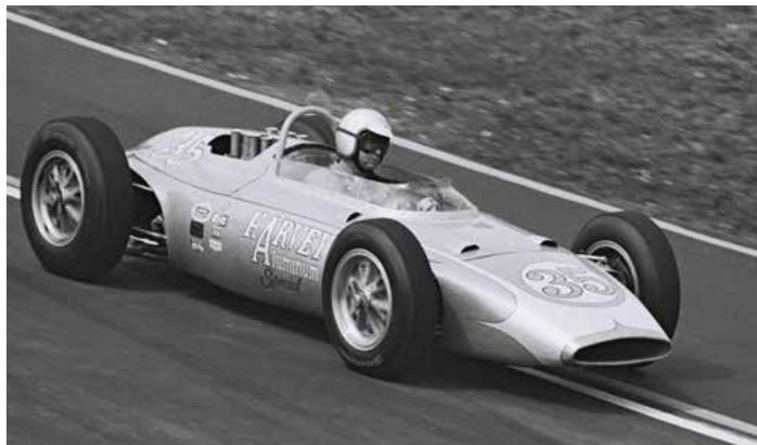
Hot rodding legend Mickey Thompson teamed up with British chassis designer John Crosthwaite to build three Buick-powered mid-engine fully independent-suspension cars for the 1962 race, all sponsored by Harvey Aluminum. While "rookie" Dan Gurney qualified eighth, but Bill failed to get the second team car up to qualifying speed before crashing. Bill was not hurt. Gurney managed 92 laps before the car blew an improperly installed grease seal in the transaxle and the gears locked up.
